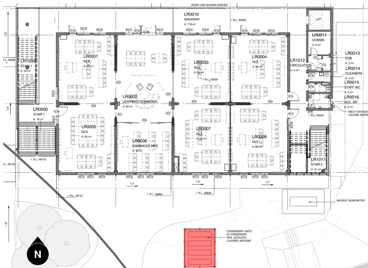
Figure 5: Proposed location of external mechanical plant (red shadow).
